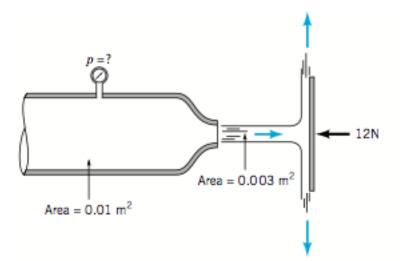
Air flows into the atmosphere from a nozzle and strikes a vertical plate as shown in the figure above. A horizontal force of 12 N is required to hold the plate in place.
