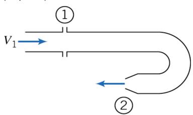
Water is flowing steadily through the 180° elbow shown above. The water discharges to the atmospheric pressure.
