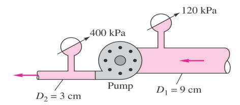
The horizontal pump in the figure discharges water at 57 m<sup>3</sup>/h. Neglecting losses, what power in kW is delivered to the water by the pump?
