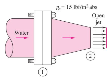
The horizontal nozzle in the figure has  $D_1 = 12$  in,  $D_2 = 6$  in, with  $P_1 = 38$  psia, and  $V_2 = 56$  ft/s. Find the magnitude of the force F (in lbf) provided by the bolts to hold the nozzle in place.
